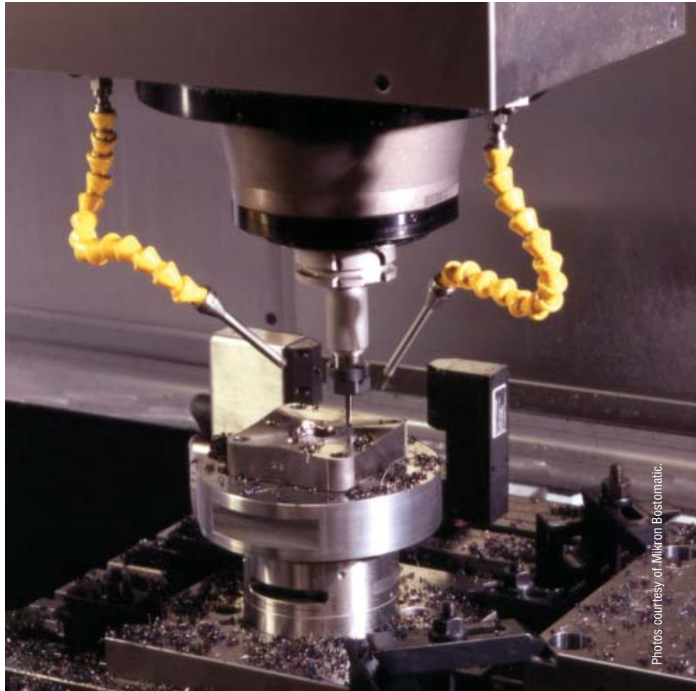
HSM eliminated costly time-consuming steps—such as 50 percent or more EDMing and hand finishing—to build the Edwards molds faster and with better precision.
